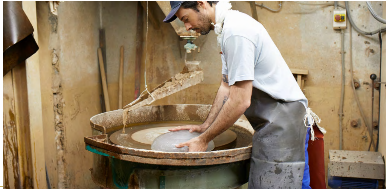
Opposite, the lapidary: the oldest station in the workshop, unchanged since the 1930s. The glassmakers continue to use this wheel, in particular to polish the edges of cut-outs in order to perfectly fit the dimensions of the lamps.
